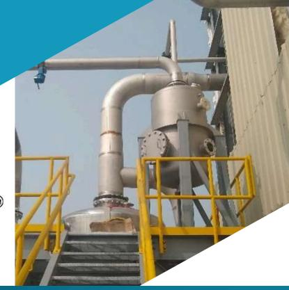
The Syrup Concentrator™ is a unique high-efficiency forced-circulation evaporation system designed to concentrate de-oiled syrup to total solids concentrations over 50% TS\*.
