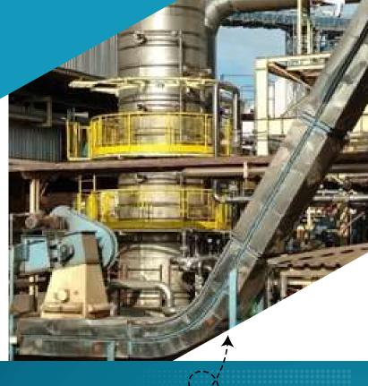
An example of an ExTactor installed on a DTDC process drying section (hexane seed oils extraction facility, South America)
